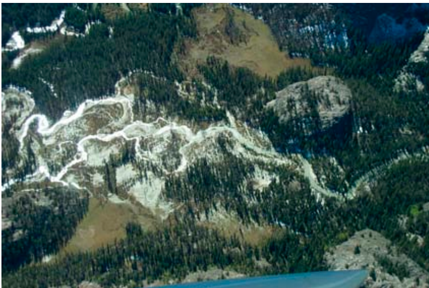
Figure 5. Aerial view of Downs Fork Meadows in late September 2003, showing extent of flood deposition in ephemeral lake, channel avulsion, and overbank flows. Left is downstream.
