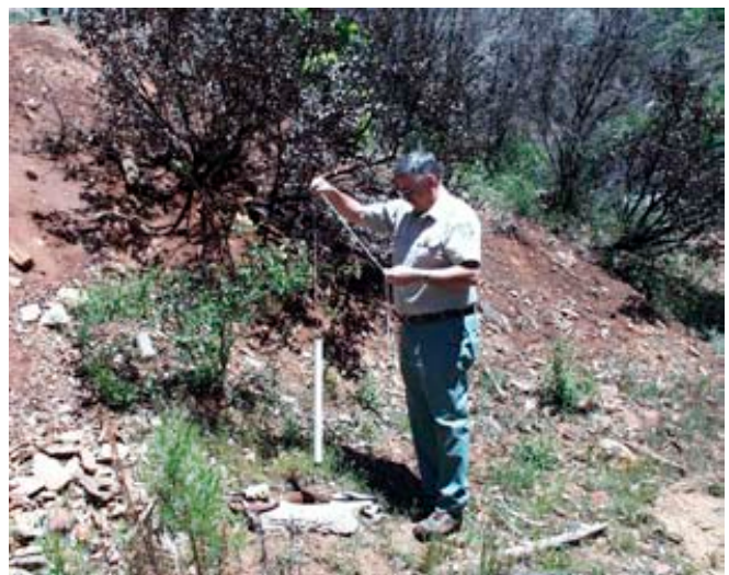
Figure 7. The senior author (DeGraff) purging monitoring well BS-45 with a bailer on the Stanislaus National Forest. A second bailer is used to collect the sample after well purging. A housing installed flush to the ground surface protects the well between sample events. See Figure 6 for details.
