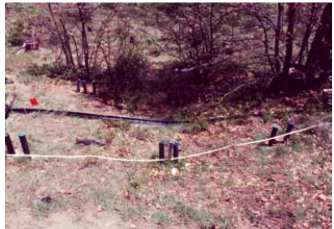
Figure 3. A view down slope from the application area toward the Class 4 channel that runs from left to right across the background. The clusters of lysimeters are visible on the boundary of the application area and buffer zone and along the line 3.1 m down slope. A black plastic barrier at 4.6 m diverts surface runoff to the surface water sampler.
