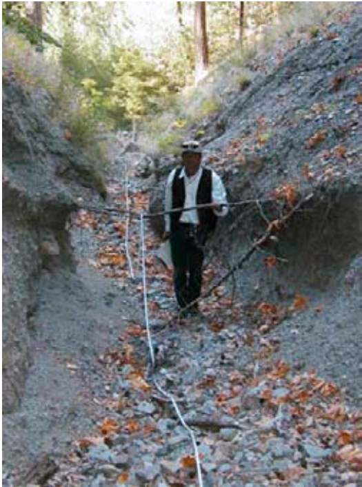
Photo 3: Incipient slope failure due to oversteepened channel side slope.
