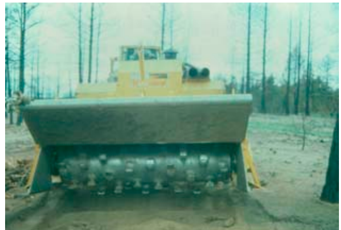
Figure 1. Rotoclear machine showing rotating drum.
