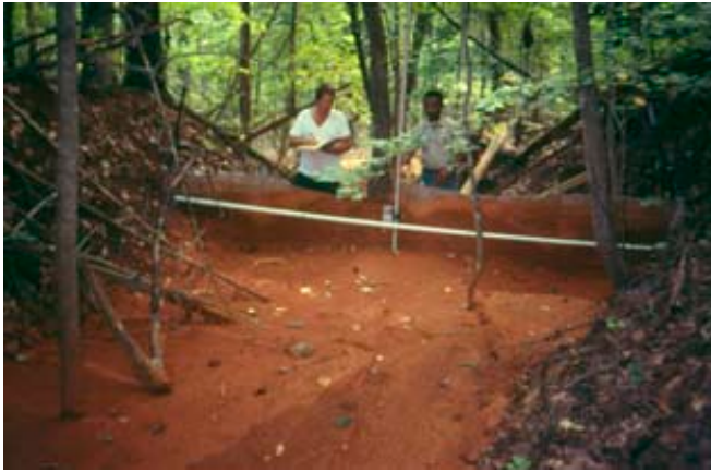
Figure 7. About 4.5 tonnes (5 tons) of sediment were deposited from Tropical Storm Beryl in August 1994. Sediment surface elevations and bulk density measurements were taken to estimate sediment amount.
