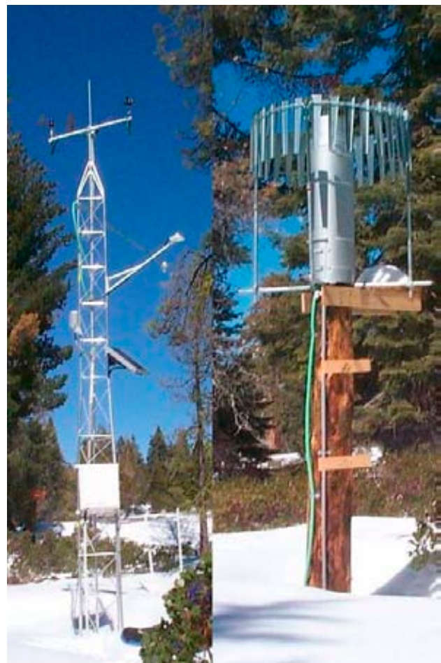
Figure 3. Sensors on a 6-meter tower at the upper Providence meteorology station measure temperature, relative humidity, solar radiation, wind speed, wind direction and snow depth (left). The 3-meter high Belford® gauge measures total precipitation (right).
