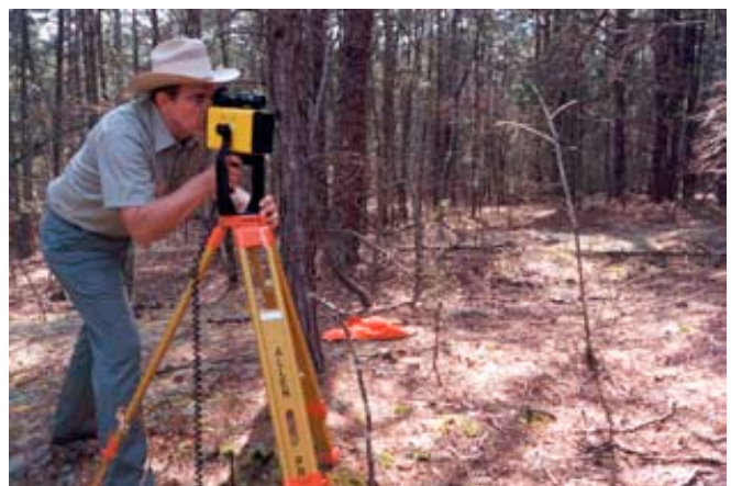
Figure 6. A Criterion 400 survey laser provided quality measurements to determine gully drainage extent. Laser has selective filter that can detect prism through vegetative cover, or can shoot directly to any solid surface, measuring distance, azimuth, slope and elevation change.
