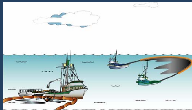
Figure 2. Typical on-water mechanical response system
