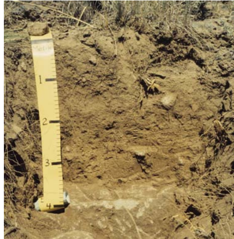
The soil is residual derived from flow andesite and is stony on the surface. Texture is stony silt loam. The 4-dm depth occurs in a 500-mm precipitation zone supporting ponderosa pine. Because the shallow soil's field capacity is exceeded, it becomes water logged in the winter and early spring apparently precluding pine establishment. Juniper occurs on fault lines.
