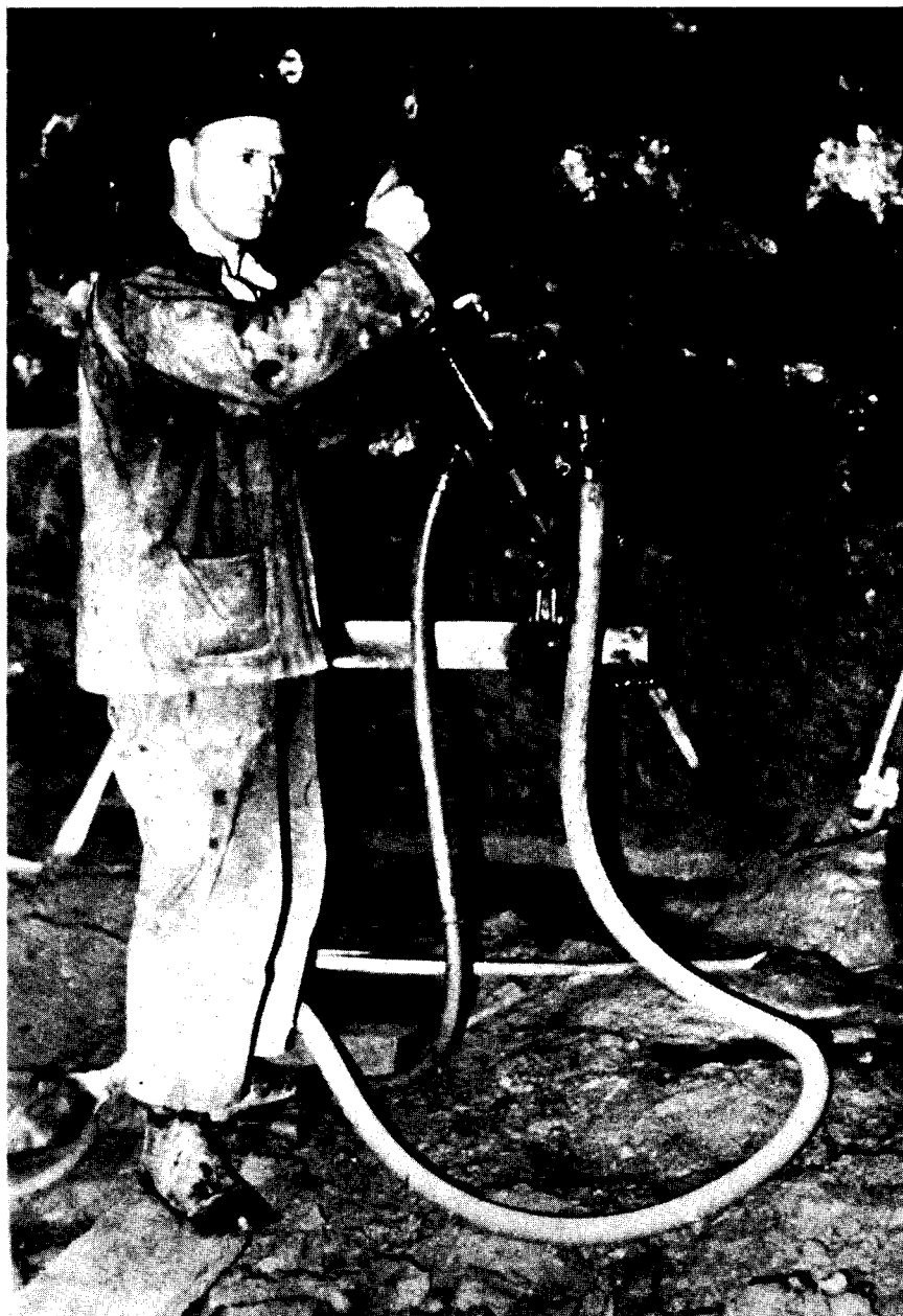
William Byington at the Alaska Juneau Mine operating a Gardner-Denver 17L drifter drill in 1941 ( courtesy of Alaska Electric Light and Power Co. )
