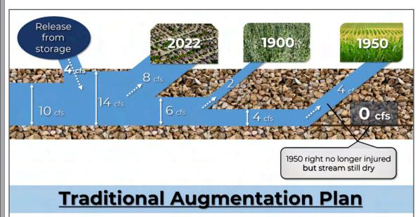
Figure 5: Fictional stream with introduction of replacement source from storage via augmentation plan
