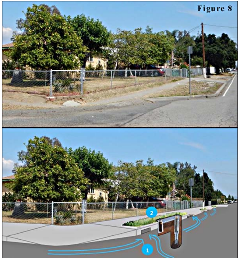
Figure 8 – Proposed Drywell Installation on Laurel Canyon Project
