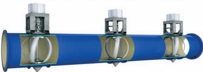
Cutaway of LucidPipe In-Conduit Generation System showing internal hydrofoils and external generators
