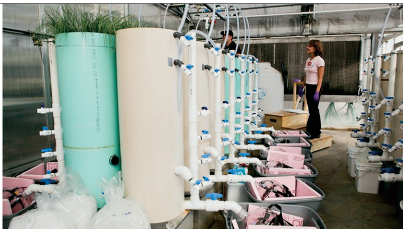
Soil Columns at WSC Filter Highway Runoff to Assess Rain Garden Efficacy
