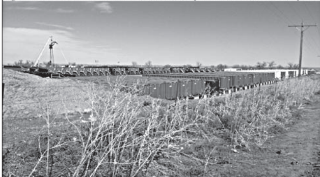
Figure 4: Additional Frac Tanks and Water necessary for a Horizontal Well Completion
