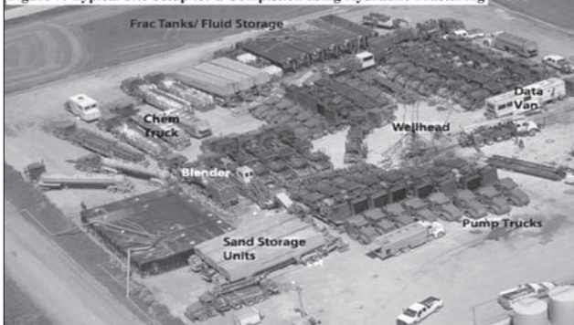
Figure 4: Additional Frac Tanks and Water necessary for a Horizontal Well Completion
