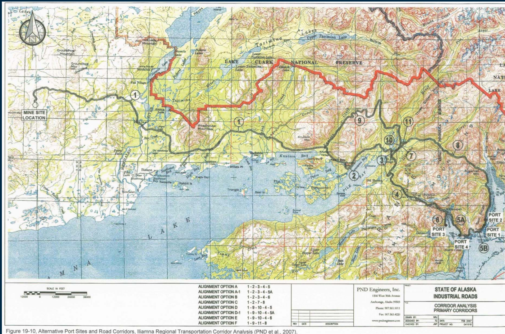
Figure 19-10, Alternative Port Sites and Road Corridors, Iliamna Regional Transportation Corridor Analysis (PND et al., 2007).
