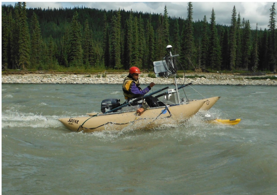
Figure 2. ADCP measurement platform.
