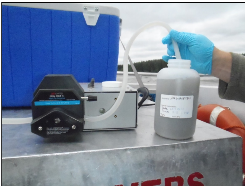
Photo I-5. Collecting non-filtered water sample using peristaltic pump
