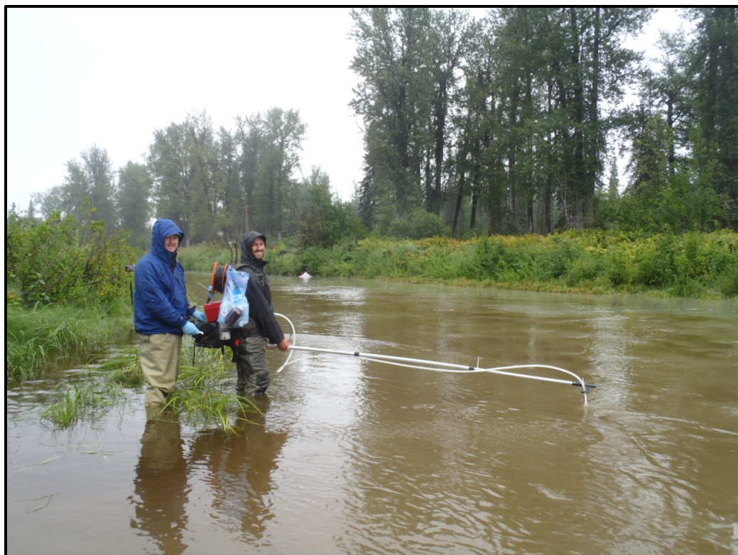
Photo I-7. Portable sampling equipment used for collection water quality samples in shallow water areas.
