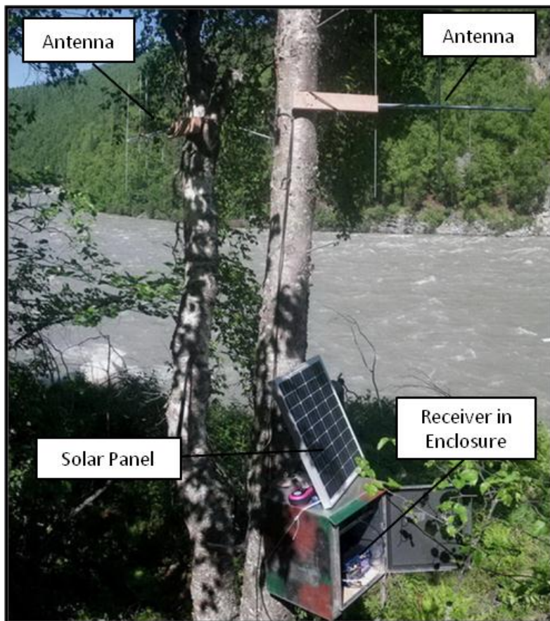
Photo 4. Fixed-station receiver site near Chinook Creek on the Susitna River, July 19, 2012.
