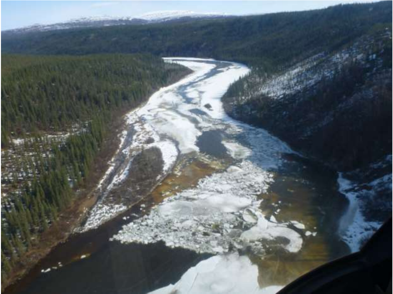
Figure 5.4-13. Ice jam at RM 231, April 27, 2012.
