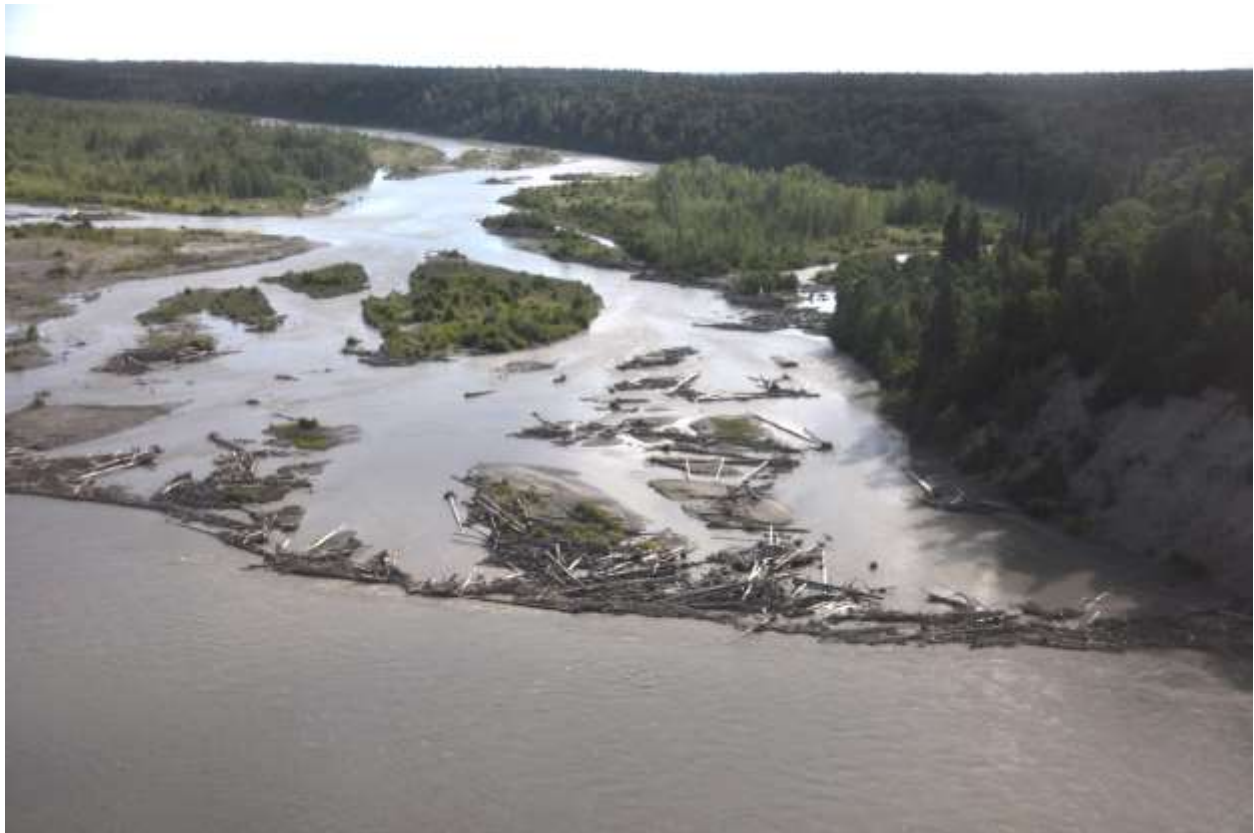
Photograph 21. June 30, 2012 Lower Susitna River between Talkeetna and Willow. Unstable accumulations of racked wood debris upon bars and stable island bar apex jams with racked members.
