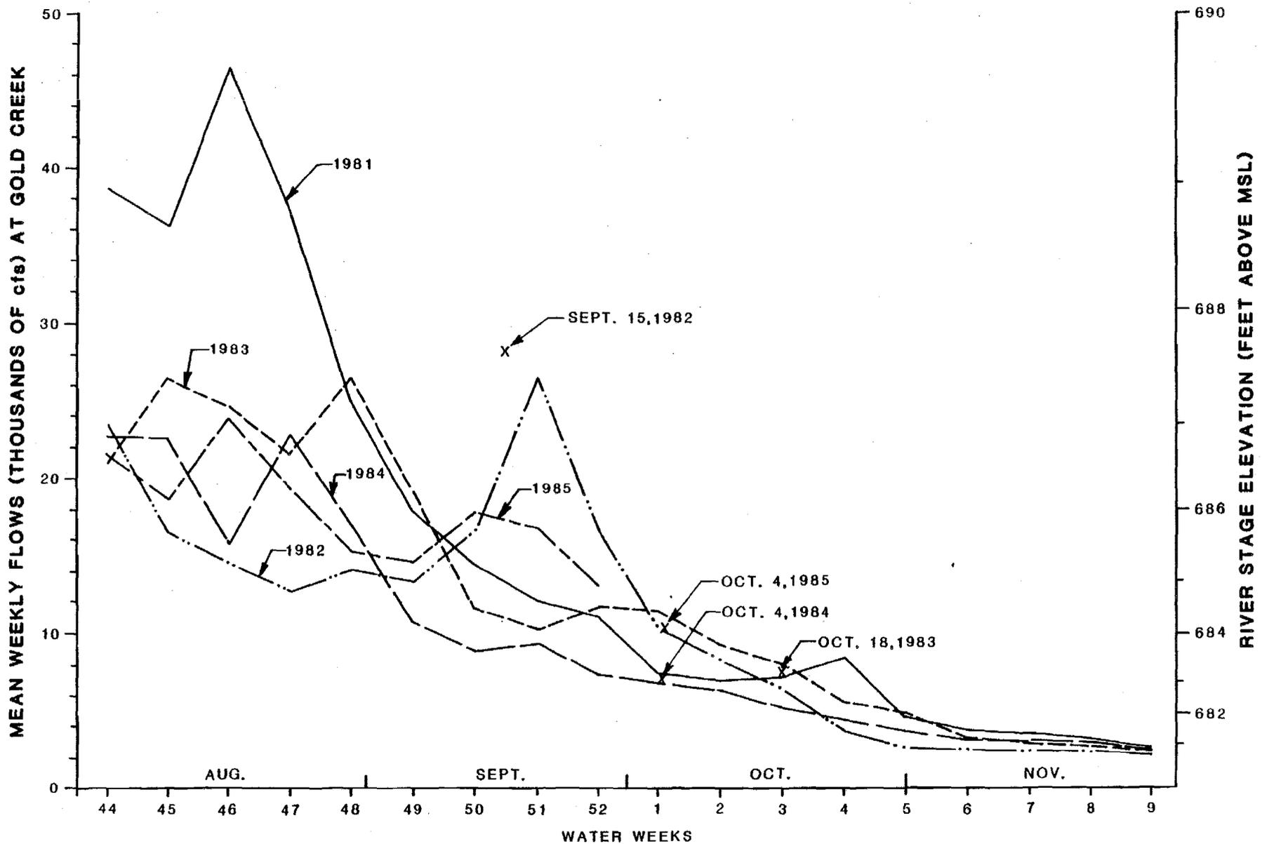
FIGURE 2. MEAN WEEKLY FLOWS AND STAGES OF SUSITNA RIVER, ALASKA, AT THE GOLD CREEK GAGING STATION DURING THE FALLS OF 1981 TO 1985. 'X's REPRESENT FLOW ON CACHE SURVEY DATES
