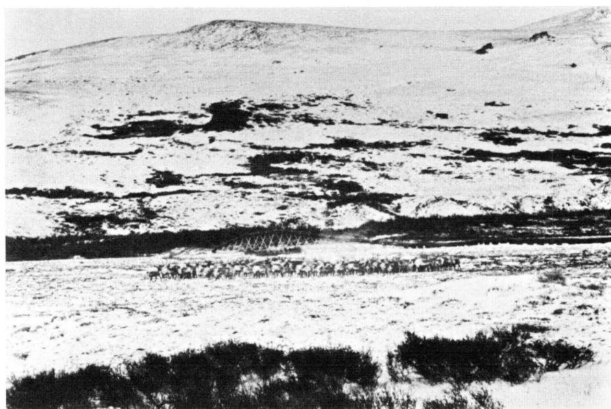
Fig. 7.—A herd of reindeer mill in close proximity to a simulated pipeline in the Penny River valley, Seward Peninsula, Alaska. The elevated section and gravel ramp constructed as experimental crossings can be seen behind the herd (Photo by D. R. Klein).
