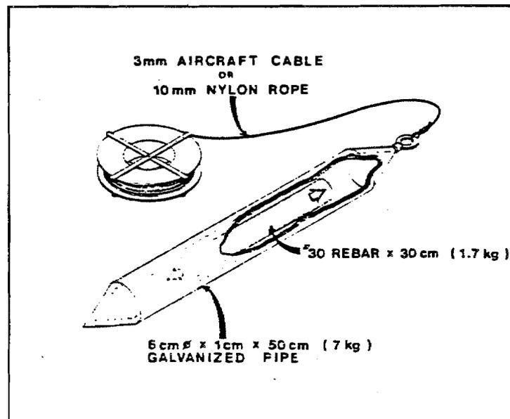
FIGURE 10 - PROBE FOR PENETRATING SLUSH ICE
