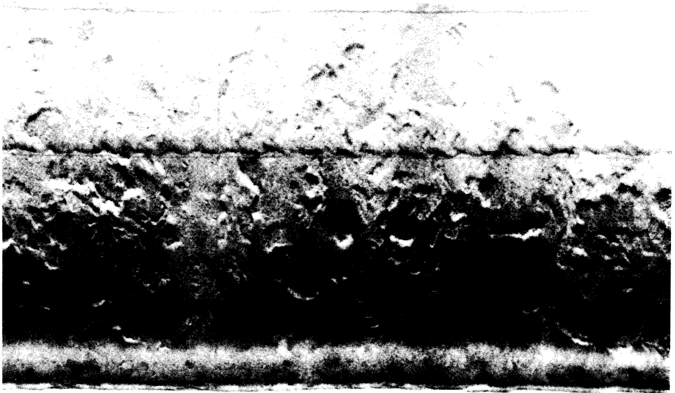
Figure 12. Bottom depressions depicted on 500 khz side-scan sonar records. Towing speed was 2.9 kts.
