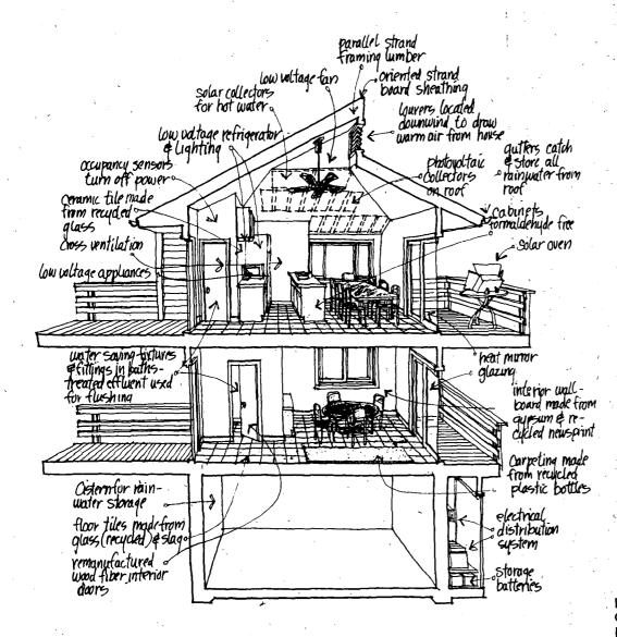
oINDEPENDENT ENERGY SYSTEM Energized by wind power and photovoltaics Applicances selected for compatibility with power Source
