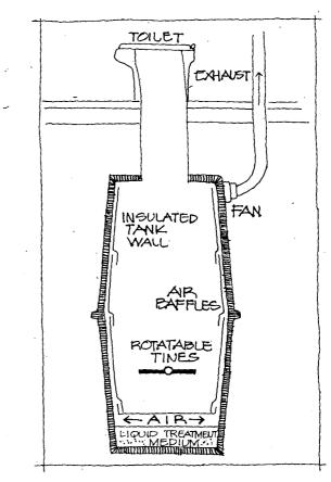
Composting toilets have several advantages over other systems — e.g., no water is used and only a small amount of energy is needed for an exhaust fan; valuable nutrients are used to benefit soils; proper maintenance requires little time.
