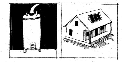
an additional heat exchanger and superinsulation. The solar collectors are generally flat-plate designs that vary from manufacturer to manufacturer. These systems are simple to install, and maintenance is low. Payback varies with comparison to local rates, but is generally two to three years.
