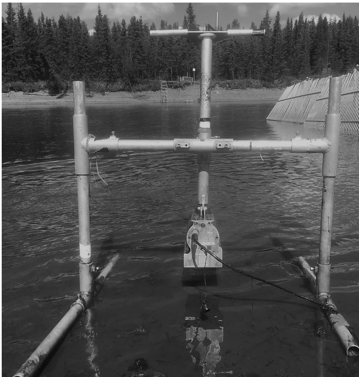
Figure 5.—View of a DIDSON mounted to aluminum H-mount with manual crank-style rotator at the Anvik River sonar project, 2017.
