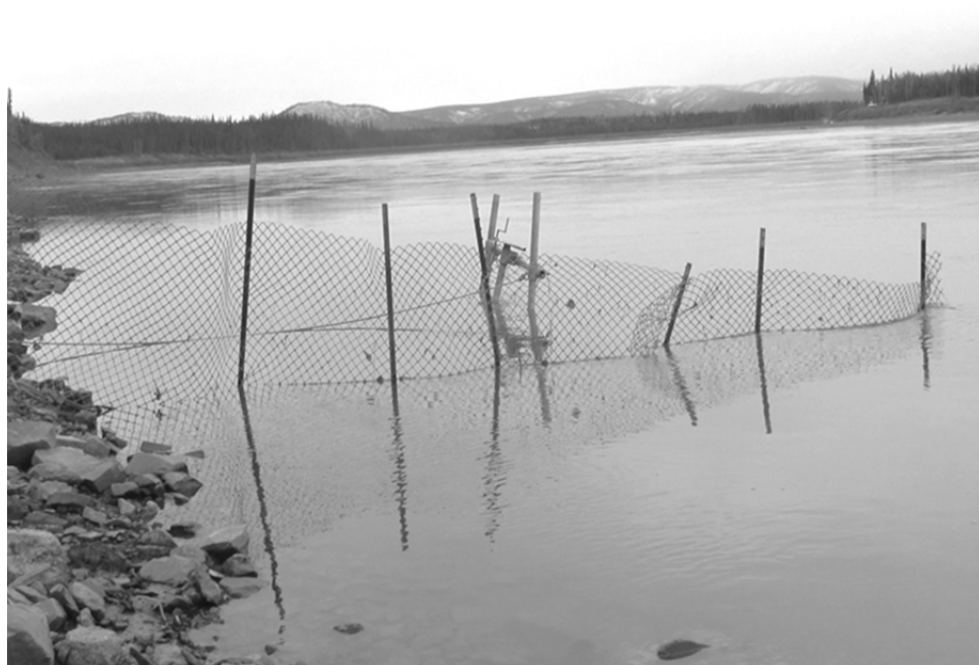
Figure 6.—Portable tripod-style fish lead used on the left bank (top) and plastic snow fencing used on the right bank at the Eagle sonar project, on the Yukon River, 2015.
