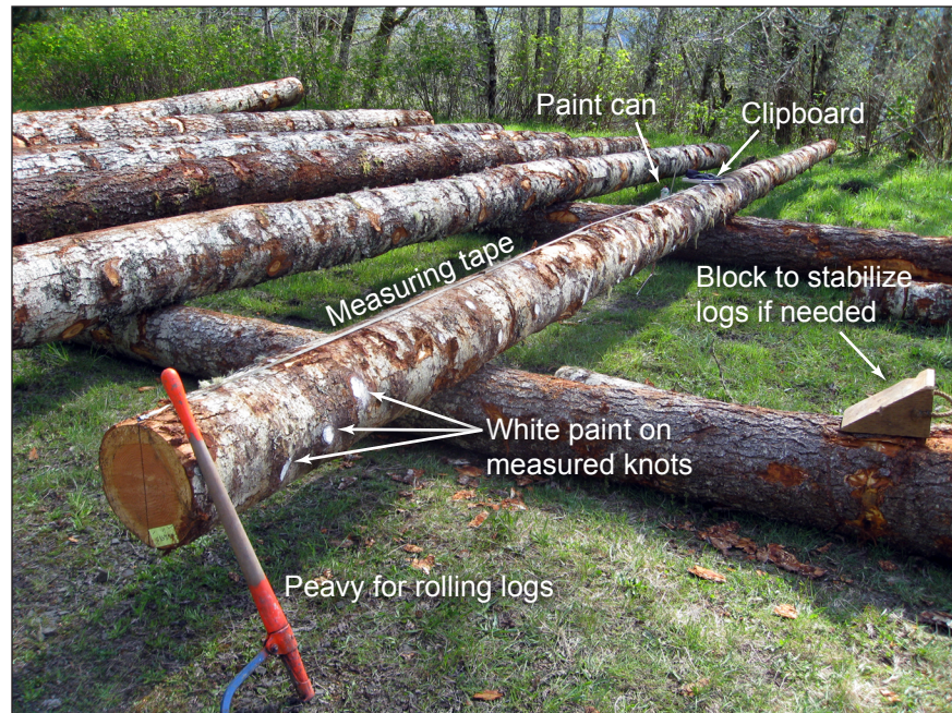
Figure 6—Stem analysis on sample logs from a sample tree harvested on Douglas-fir stands in the Oregon Coast Range 15 years after habitat-improvement thinning treatments. Data were recorded along the full length of each log in an initial ( 0^\circ ) orientation, then the log was rolled 180^\circ and defects not visible in the initial orientation were measured and recorded.
