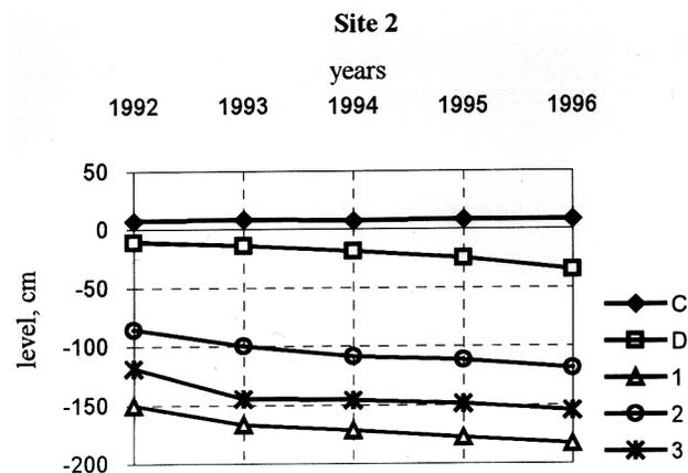
Figure 3. Surface subsidence of survey points within site 2. C: undisturbed inter-alas terrain; D: incipient thaw depression; 1-3: centers of polygons within thaw depression.
