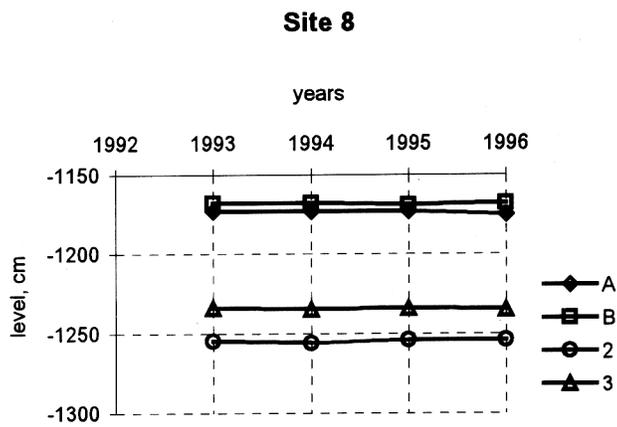
Figure 5. Surface subsidence of survey points within site 8. A and B: forested inter-*alas* terrain; 2 and 3: centers of thaw depression.
