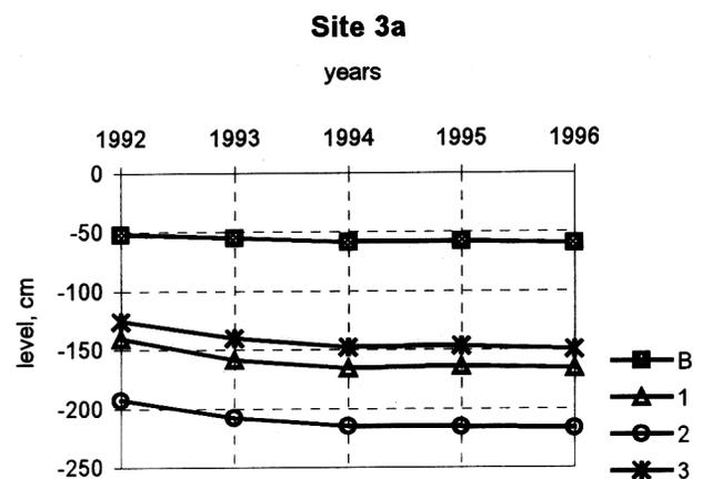
Figure 4. Surface subsidence of survey points within site 3a. B: inter-alas terrain; 1 and 3: centers of polygons within thaw depression; 2: interpolygonal trough.
