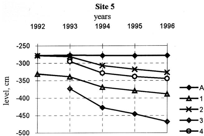
Figure 2. Surface subsidence of survey points within site 5. A: undisturbed inter-alas terrain; 1 and 2: polygon centers at the water edge; 3: polygon center, below the water edge since 1994; 4: interpolygonal trough at 5 m from the water edge.
