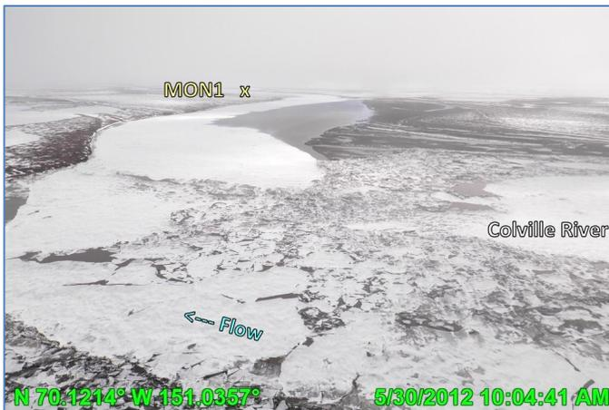
Photo 4.9: Ice jam upstream of MON1 grounding out with stage recession, downstream end looking downstream (south); May 30, 2012
