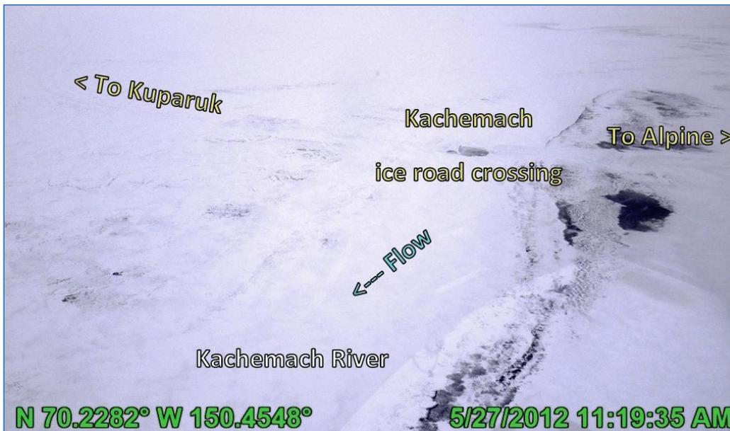
Photo 2.16: Kachemach River ice bridge crossing slotted to facilitate flood flow prior to breakup, looking upstream (south); May 27, 2012
