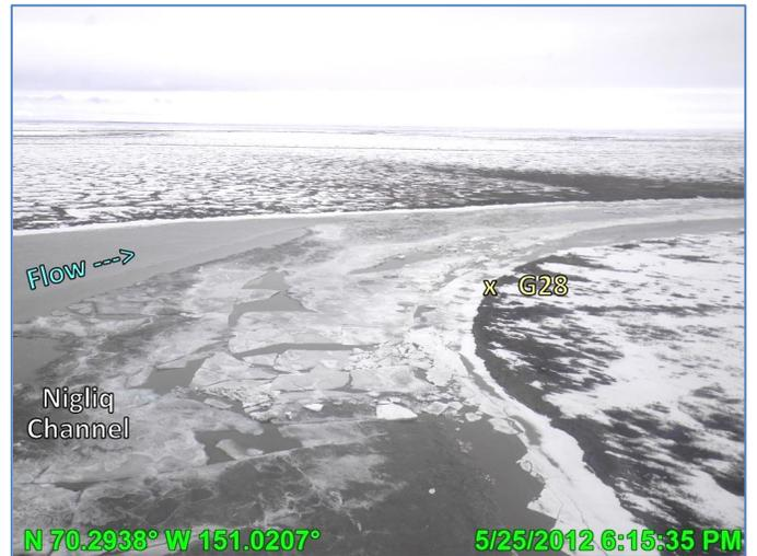
Photo 4.80: Rafted ice upstream of the Nigliq bridge location as initial flow moves through, looking west; May 25, 2012
