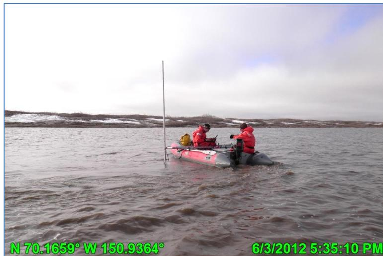
**Photo 5.1: Crew preparing to perform a direct discharge measurement at MON1 with the ADCP; June 3, 2012**
