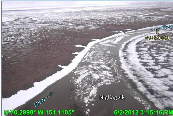
Photo 4.88: Ice jamming in the Nigliagvik at the crossing location prior to peak stage, looking downstream; June 2, 2012
