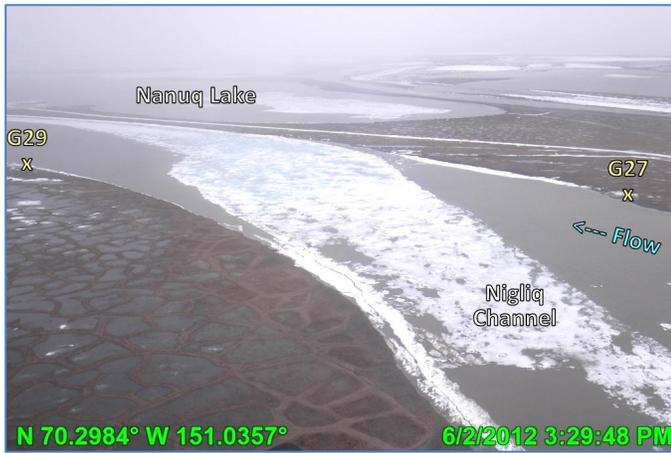
Photo 4.86: Channel ice rotting just prior to peak stage at the Nigliq bridge location, looking downstream (northeast); June 2, 2012
