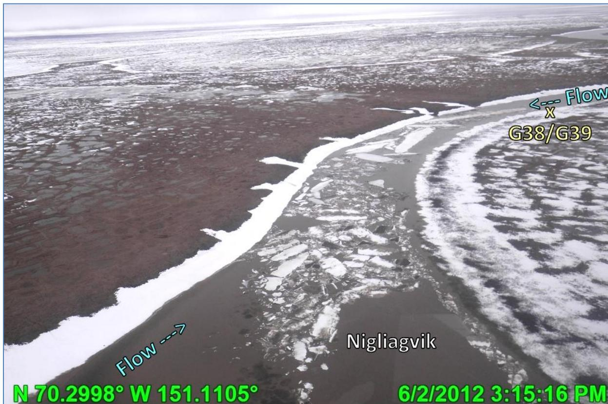
Photo 5.6: Ice jam in the Nigliagvik during peak discharge, looking downstream (north); June 2, 2012
