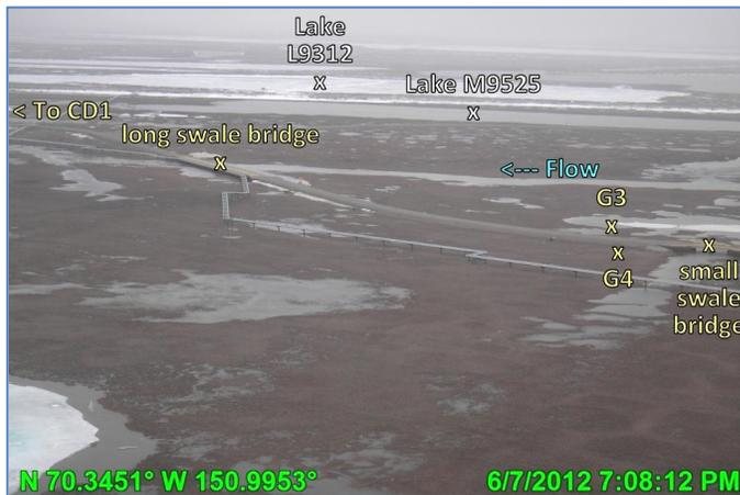
Photo 4.48: Limited flow through the long swale bridge and ponded water at the short swale bridge as stage recedes at G3/G4, looking south; June 7, 2012
