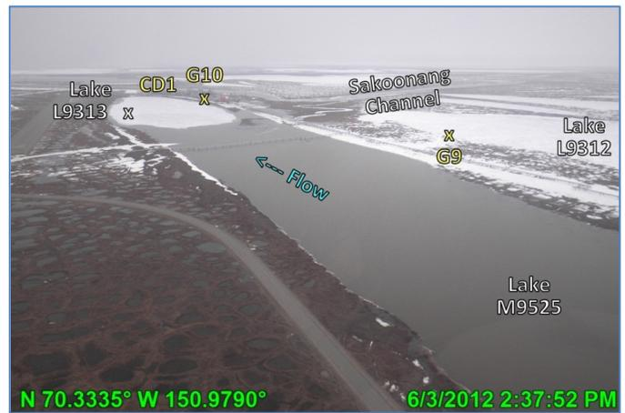
Photo 4.56: Lake L9313 receiving additional recharge from the Sakoonang prior to peak stage; no melt or overland flow into Lake L9312, looking east; June 3, 2012
