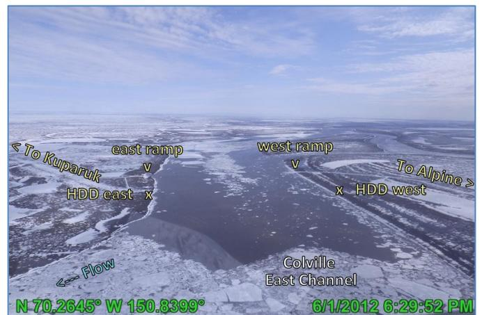
Photo 4.66: Colville ice bridge gone as jam release from upstream of MON1 passes through, looking upstream; June 1, 2012
