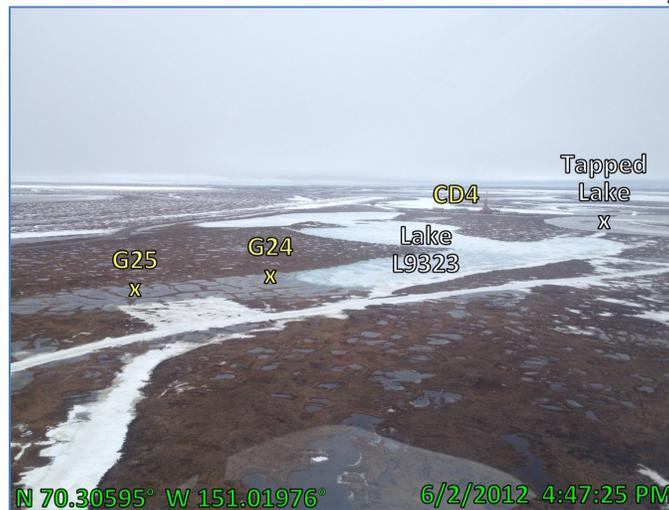
Photo 4.83: Stage was not high enough in the Nigliq during peak to overflow into Lake L9323 resulting in local melt only at crossing location, looking south; June 2, 2012
