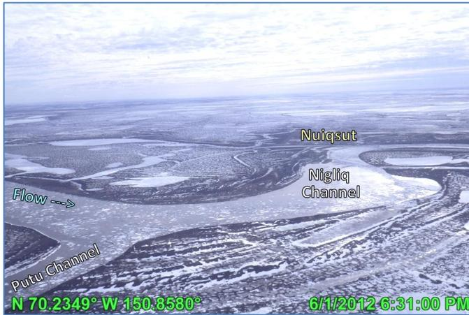
Photo 4.22: Floes from a jam release upstream of MON1 diverting into the Nigliq to contribute to the ice jam adjacent to Nuiqsut, looking west; June 1, 2012
