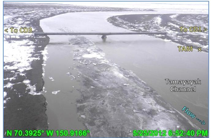
Photo 4.71: Low velocity flow in the Tamayayak moving downstream past the pipe bridge gages, with rafted ice, looking upstream (east); May 25, 2012
