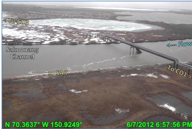
Photo 4.76: Recession at SAK gages, looking northeast; June 7, 2012
