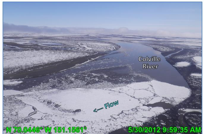
Photo 4.10: Ice jam upstream of MON1 grounding out with stage recession with non-inundated upstream overbanks, upstream end looking upstream (south); May 30, 2012
