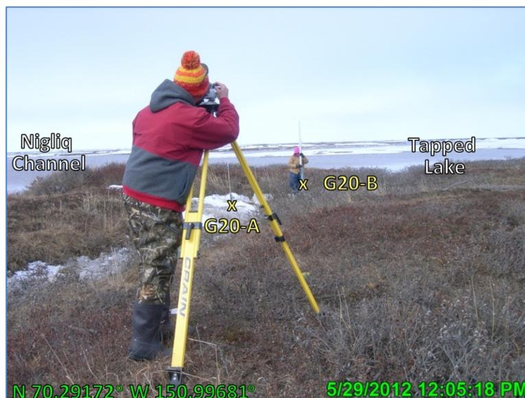
**Photo 3.4: Surveying temporary indirect-read gages (G20) to BPMSL elevation; gage A is nearest to the channel centerline; May 29, 2012**
