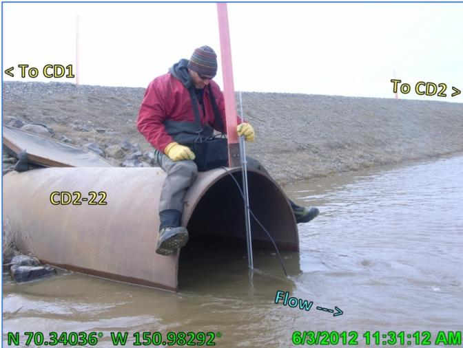
Photo 4.41: Discharge measurement at CD2 road culvert CD2-22, performing as designed to pass sediment laden flow, downstream (north) side; June 3, 2012
