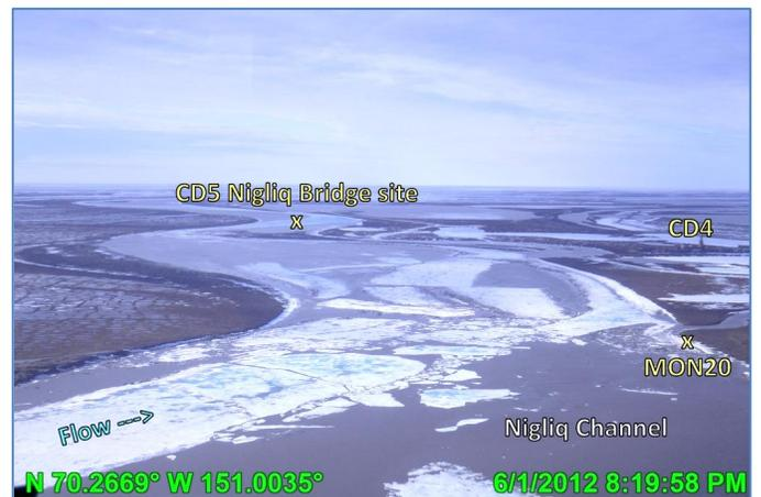
Photo 4.21: Ribbon ice through MON20 reach disintegrating into floes which accumulated upstream of the proposed CD5 Nigliq Bridge location, looking downstream (north); June 1, 2012
