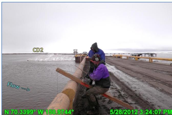
Photo 5.7: Discharge measurement at the long swale bridge, looking west; May 28, 2012
