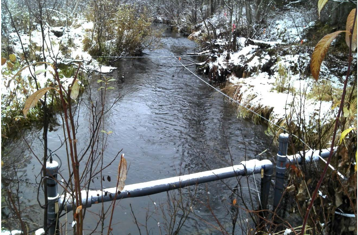
Figure 9. Buddy Creek PIT tag antennas shown with taped measured cross-sections in October 2014, looking downstream
