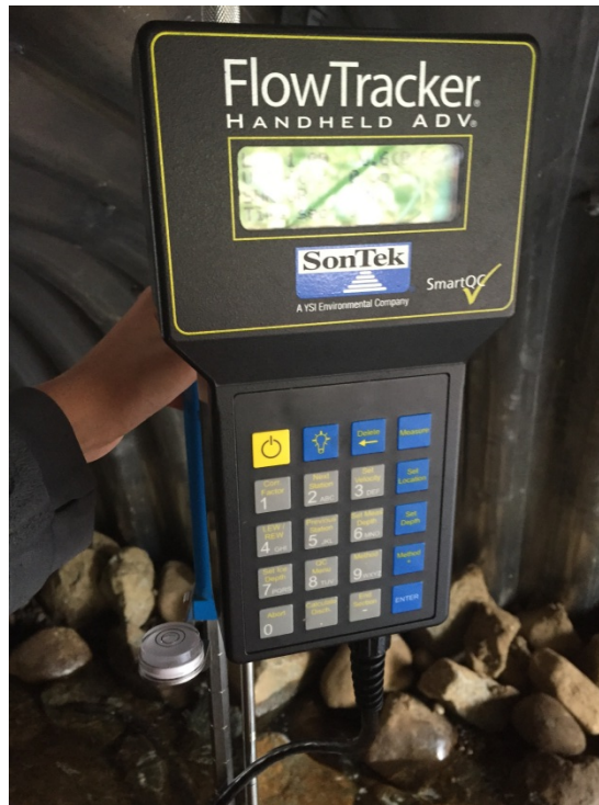
Figure 11. ADF&G-owned ADV used for measurements
