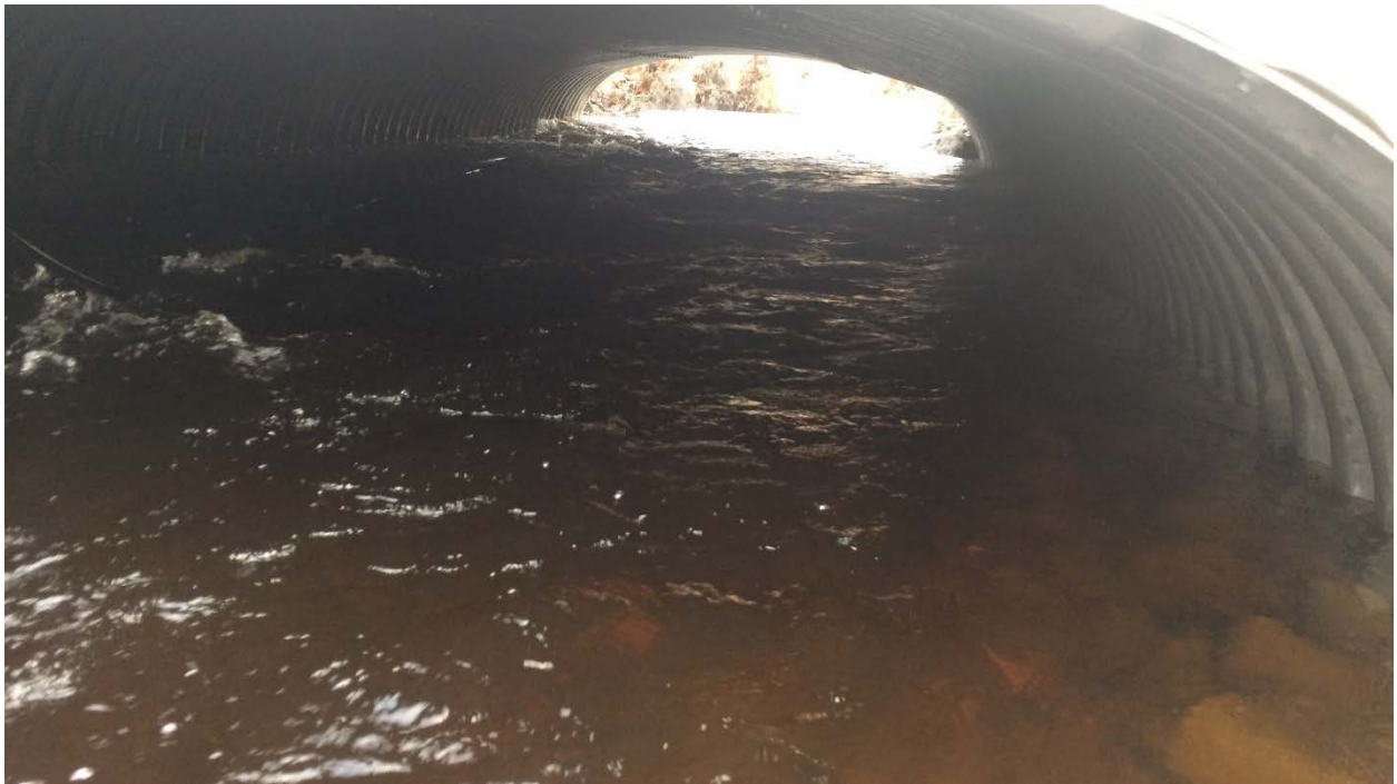
Figure 25. Flow inside arch culvert at Q=90 cfs
