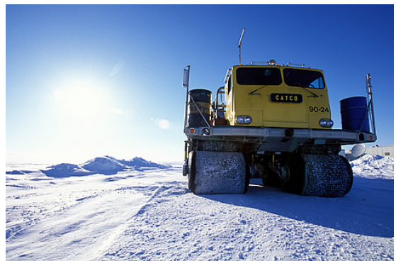
Figure 1: Rolligon all-terrain vehicle on the North Slope use low-pressure, adjustable tires to compact snow without damaging tundra (National Energy Technology Laboratories n.d.)
