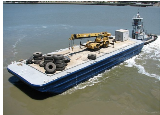
Figure 4: A deck barge can be used for equipment transport or can function as a floating work surface for subsea construction (Jerico Products, Incorporated 2010).
