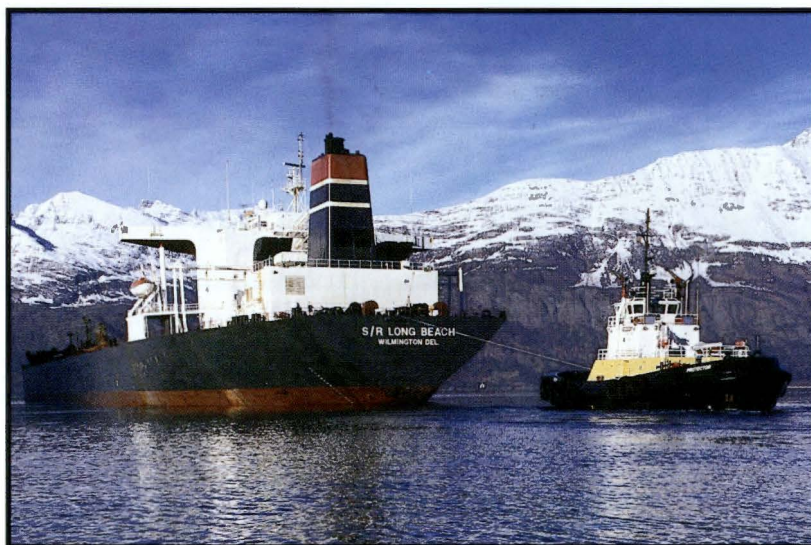
The tractor tug Protector is tethered to its charge, the SeaRiver Long Beach, for the first part of the tanker's journey out of Prince William Sound. The upgrading of escort vessels and escort practices is one of the most significant safety improvements of the last decade. Photo: Patrick C. Welch.
