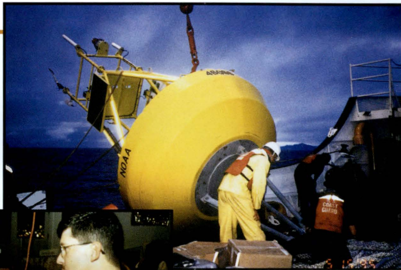
Weather buoys installed in Prince William Sound in 1995 provide more accurate and timely information about wind and sea conditions. Photo: Vince Mitchell.
