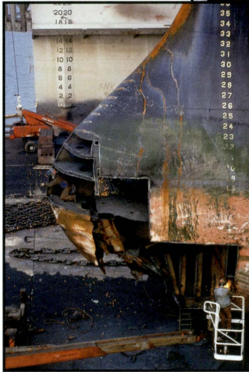
◀ The Overseas Ohio suffered major damage when it struck an iceberg in 1994. The tanker was not carrying crude oil at the time. Photo: Port of Portland.
