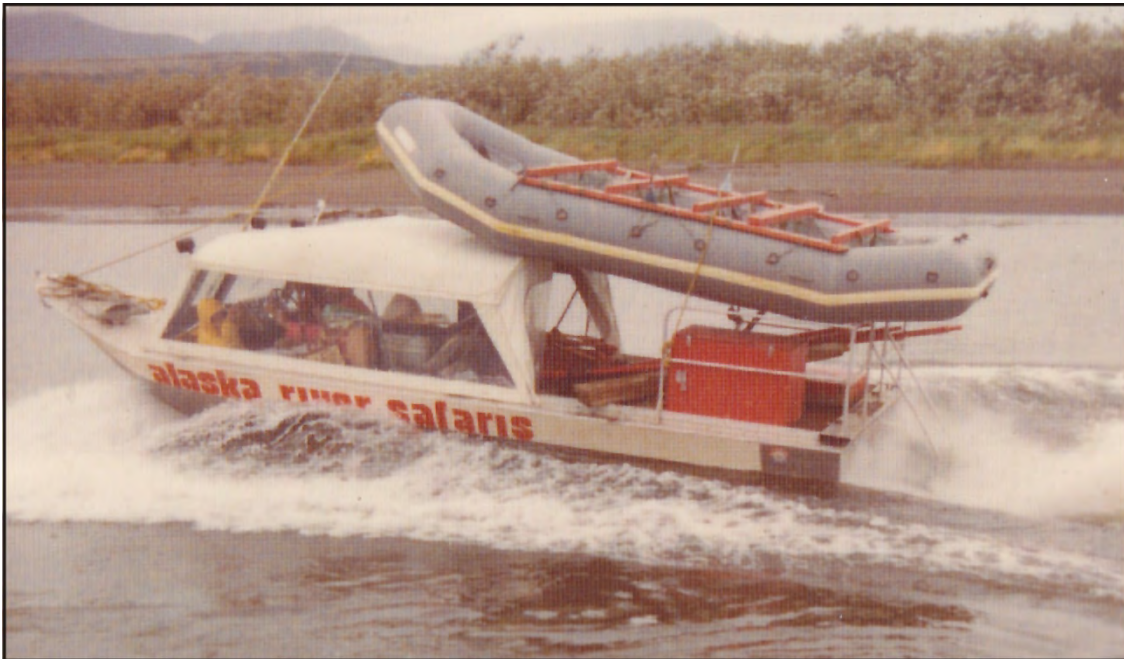
Figure 18. Hauling a raft up the North Fork on a 25-foot Duckworth jet boat with a 454-cubic inch Chevy engine and 3-stage Hamilton inboard jet, in the late 1970s.
