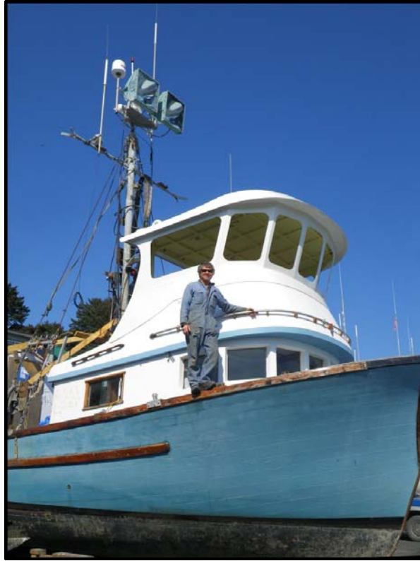
Figure 7-9 Newly Constructed Pilothouse
