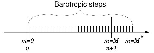
Figure 5: The split time stepping used in the model.
