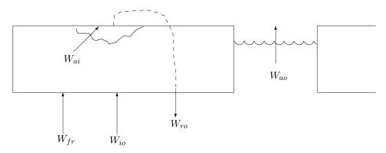
Figure 7: Diagram of the different locations where ice melting and freezing can occur.
