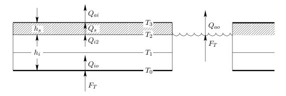
Figure 8: Diagram of internal ice temperatures and fluxes. The hashed layer is the snow.
