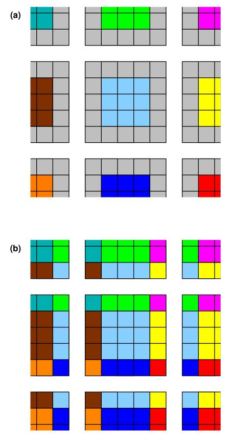
Figure 16: A tiled grid with out-of-date halo regions shown in grey and the interior points color-coded by tile: (a) before an exchange and (b) after an exchange.
