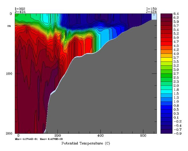
Figure 24: Vertical slice if temperature, averaged over the month of April, 1959. The slice is across the Bering Sea shelf, showing the transition from vertically mixed at the coast, a two layer system at mid-shelf, then a thermocline over the shelf-break.
