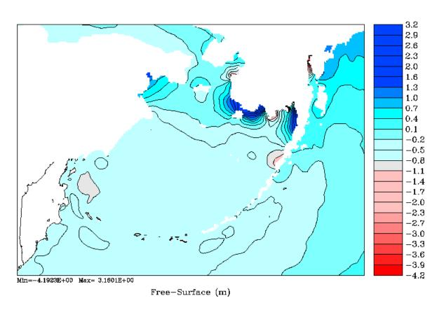
Figure 22: Surface elevation after 200 days showing tides. This is from a snapshot in a history file—the averages files have been detided.
