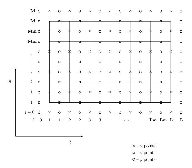
Figure 12: The whole grid. Note that there are **Lm** by **Mm** interior computational points. The points on the thick outer line and those outside it are provided by the boundary conditions.
