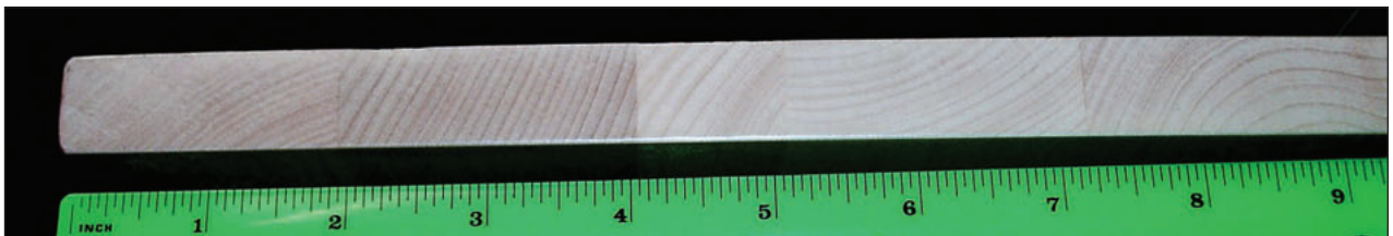
Figure 2—Panel warpage can be controlled when growth rings in adjacent strips are oriented in random directions, as seen in this edge-glued panel from birch.
