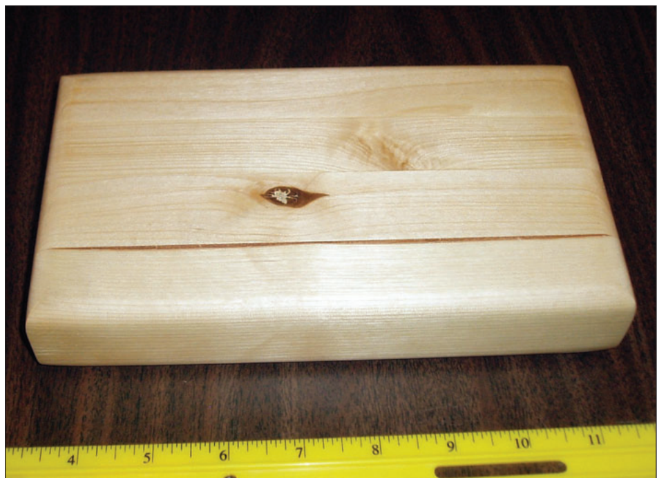
Figure 8—Edge-glued Alaska birch can be used to make craft products, such as this cutting board. Character-mark features visible above include a thin region of natural stain, a knot, and grain variation.
