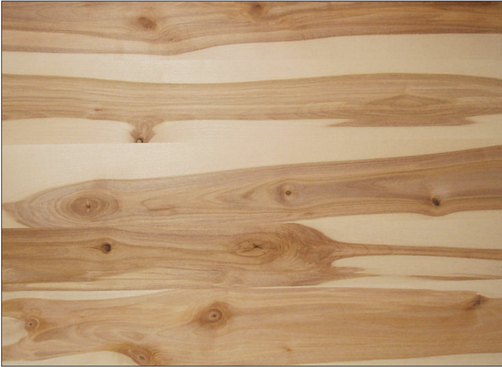
Figure 3—An edge-glued panel constructed from birch lumber containing knots and natural stain.
