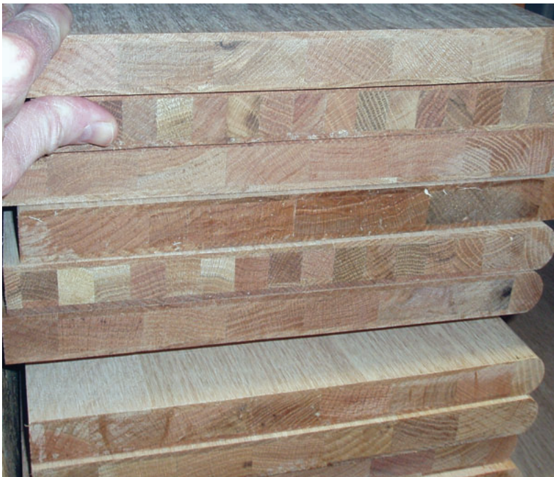
Figure 10—Stair treads are a high-value product that can include edge-glued lumber. Above, oak edge-glued laminates are enclosed in thin veneers, which form the top and bottom surfaces.
