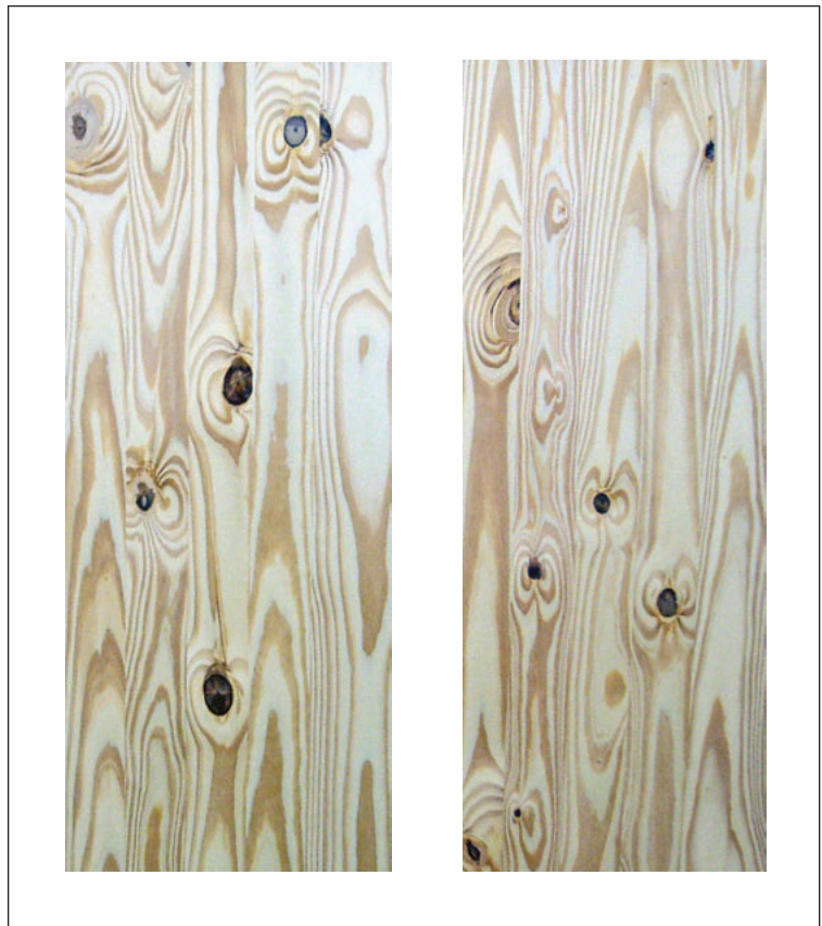
Figure 1—Edge-glued panels are often manufactured to standard dimensions. These pine panels include high levels of character such as knots and grain variation. (Photos by David Nicholls)
