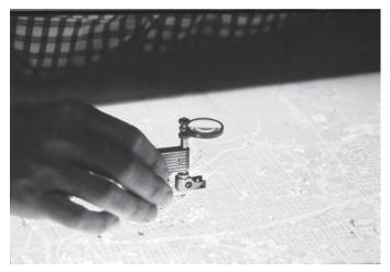
**Figure 24.** The scribing method of map production supplanted pen-and-ink drafting in the mid-1950s and produced a more legible map in a shorter time, and at less cost.
