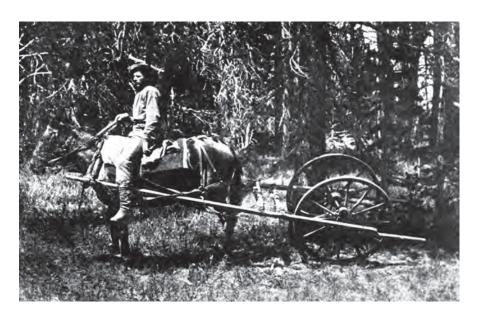
**Figure 2.** The Odometer was used to measure distance traveled by counting the revolutions of a wheel (1871).
