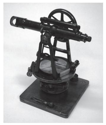
**Figure 3.** The Berger theodolite was a precision instrument used for measuring horizontal and vertical angles. Manufactured by C.L. Berger & Sons, Boston (circa 1901).
