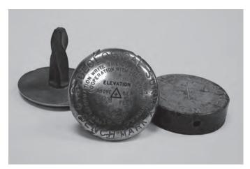
Figure 14. Bench marks were established with bronze-stemmed disks (left and middle) and caps (right) were stamped with a rounded elevation and placed by U.S. Geological Survey survey crews.
