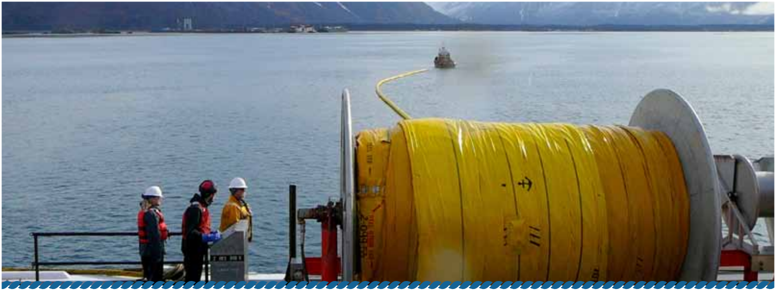
↳ A fishing vessel pulls oil-spill boom off a reel during a training exercise near Valdez. Photo by Jeremy Robida.
