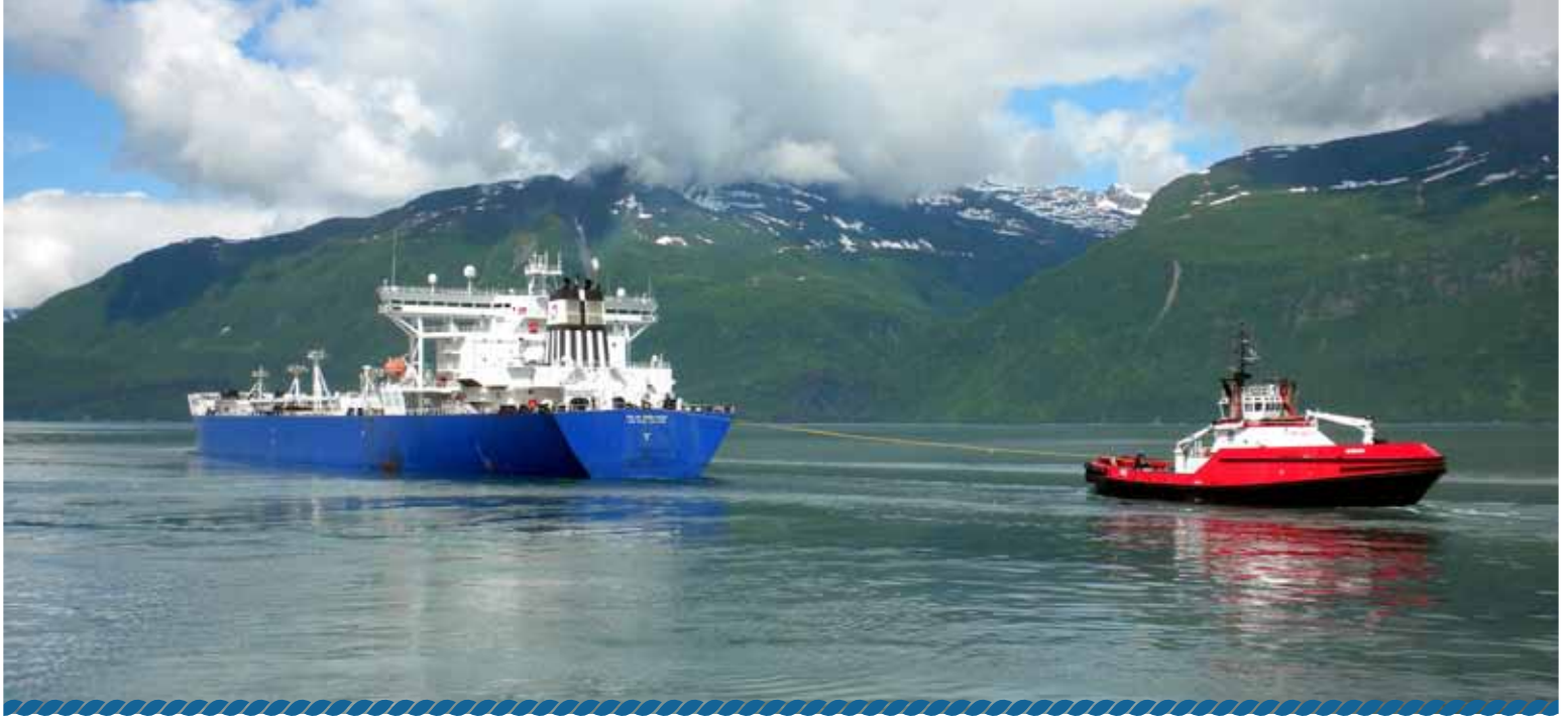
↳ The escort tug Nanoq is tethered to the stern of the tanker Polar Endeavor as it travels out of Prince William Sound with a load of oil. This photo was taken from the tanker's other escort tug. Photo by Tom Kuckertz.
