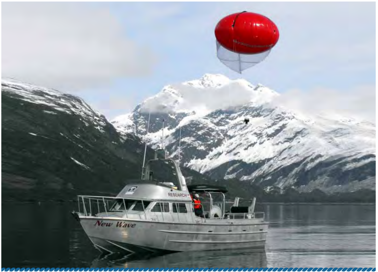
↳ Balloon-borne aerial cameras may someday be used for monitoring oil-spill response. The system shown here was tested in Cordova and demonstrated in Valdez during the summer of 2011. Photo by Donna Schantz.
