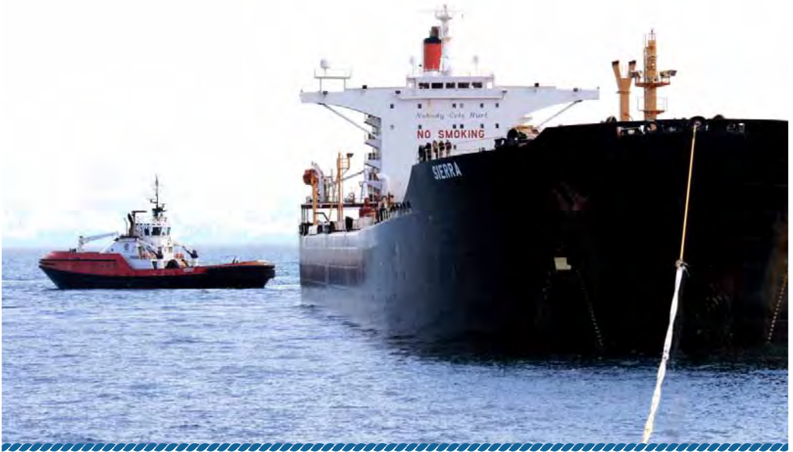
↳ The escort tug Tan'erliq is tethered to the stern of the oil tanker Sierra during a towing exercise in Prince William Sound. Photo by Alan Sorum.
