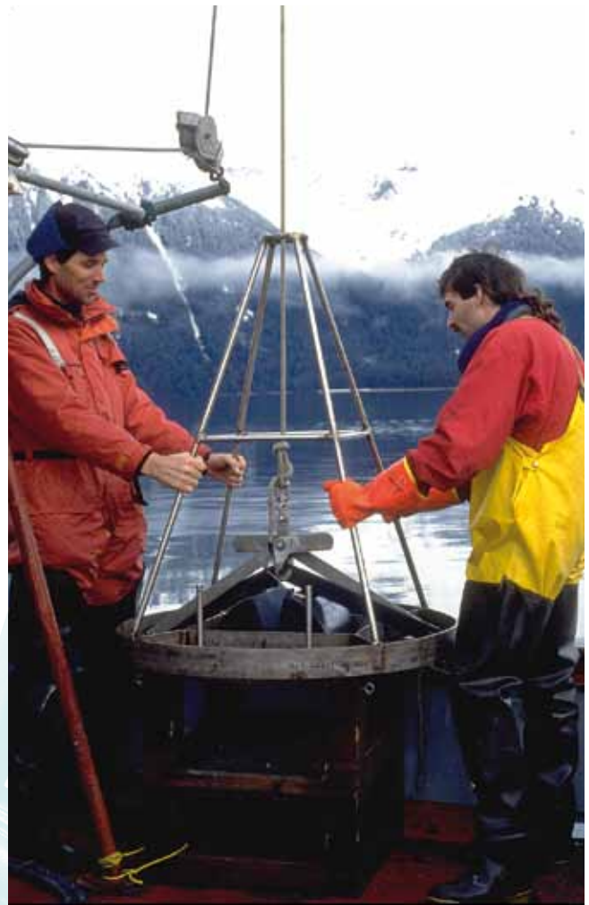
Council contractors prepare to lower a grab sampler into the water to take bottom sediment samples as part of the council's Long-Term Environmental Monitoring Program.
