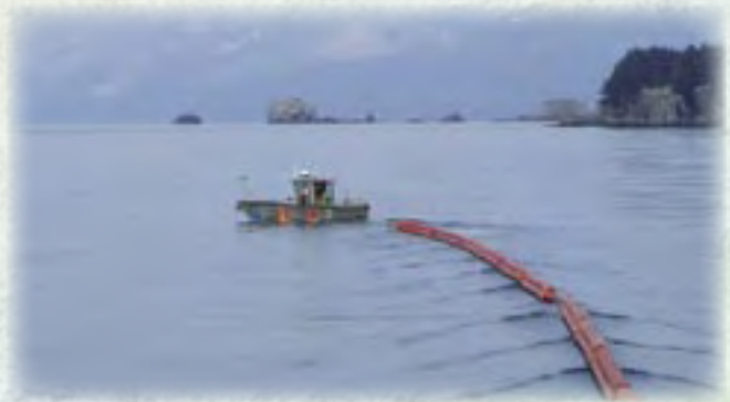
This boat pulls protective boom into place during a Geographic Response Strategy training exercise near Hinchinbrook Entrance, where loaded tankers pass out of Prince William Sound. Photo by Dan Gilson.
