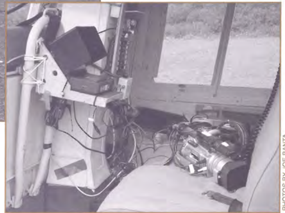
The ShoreZone mapping project uses a helicopter as an aerial camera platform to photograph shorelines (left). The system (below) includes a video camera and a computer for storing data.
