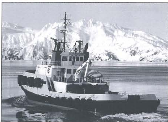
The Alert is one of a new class of powerful tanker escort vessels called Prevention and Response Tugs, or PRTs.
