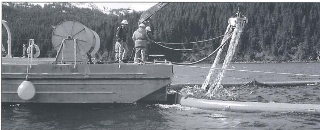
An oil-recovery device called a rope mop skimmer is deployed during a drill in Kachemak Bay in April 2000.
