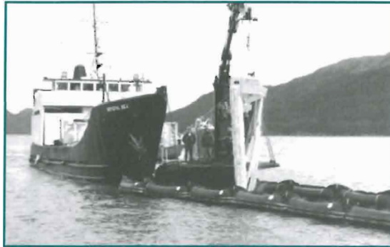
Periodic spill drills and exercises ensure that equipment works and that crews know how to use the various equipment. Here, rope mop is deployed while the Krystal Sea stands by.
