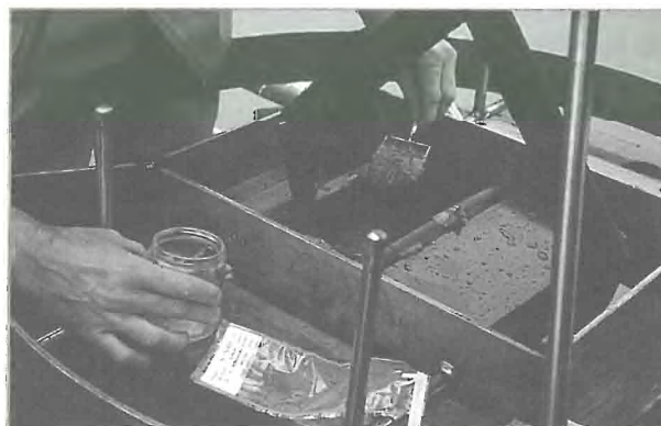
Deep water sediment samples are collected and analyzed for markers that would indicate hydrocarbons.
