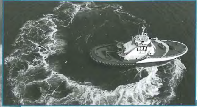
(above) Computer simulations looked at the assist capabilities of different types of tugs, including tractor tugs, which are noted for their maneuverability.
