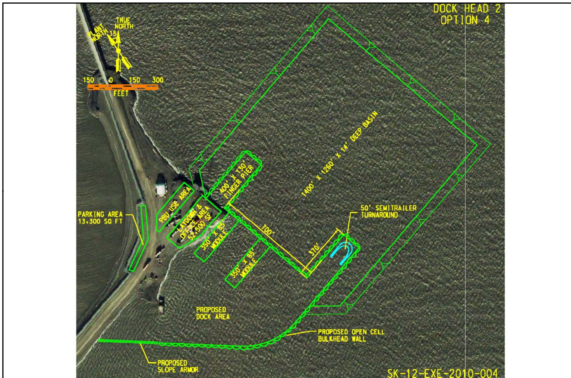
Appendix 10B Alaska Pipeline Project Dock Configuration 4
