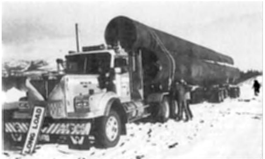
Self-steering tractor-trailer loaded with 23-m (76-ft.) lengths of pipe for test runs along the Alaska Highway.
