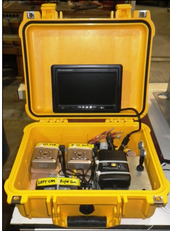
Figure 6.—Camera weir video recording components housed in a waterproof Pelican case. (©2012 ADF&G/Photo by Raymond F. Vinzant.)
