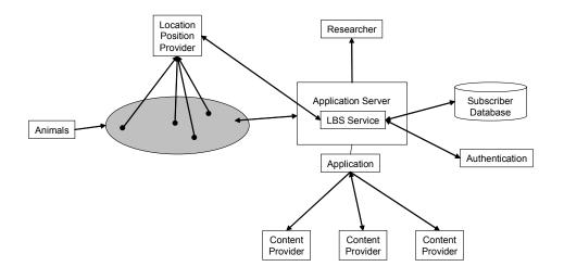
Figure 1. Wildlife telemetry LBS architecture, as adapted from Schiller and Voisard (2004).
