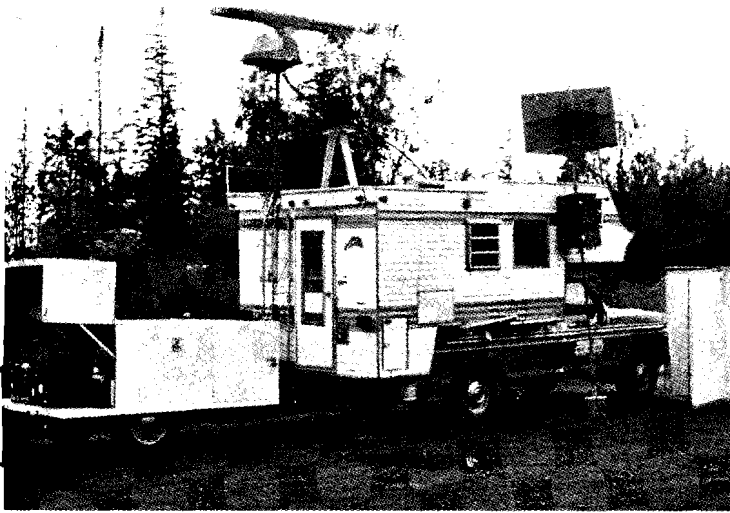
RADAR WATCH — A camper-mounted generator and radar unit was used to plot flow and circulation patterns in Kachemak Bay and lower Cook Inlet to determine the potential movement of oil pollution.
