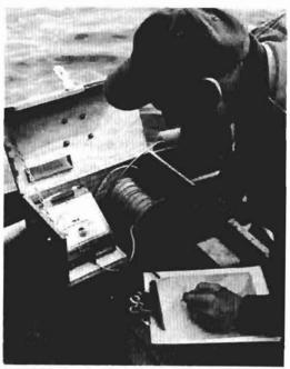
What fish scales don't say about the environment, instruments do. The temperature at various depths, and the locations of the "thermoclines"—sharp divisions between one temperature range and another—are important to a fish. This electronic thermometer helps pinpoint these areas.
