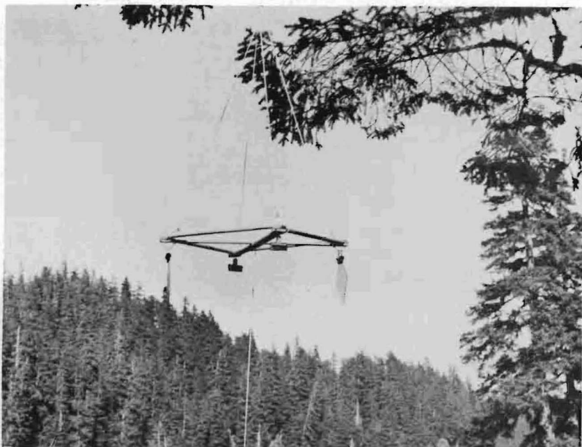
Figure 2. Glass plates suspended under surface may show lake productivity by measuring growth of attached algae.
