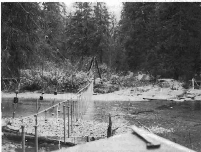
Figure 8. View of the electric weir used at Reflection Lake showing the electrodes, ground line, and in the background the holding pen.
